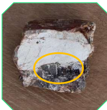
Visible cassiterite in drill core at Kalayi
