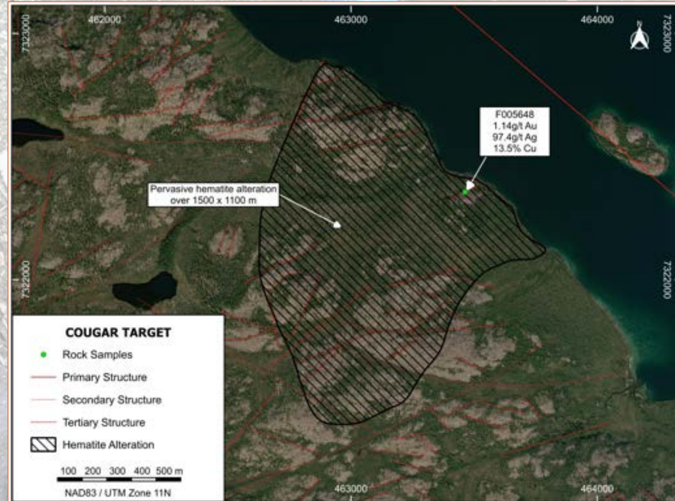
Map of the Cougar target illustrating the widespread pervasive hematite alteration and location of sample F005648 which returned 1.14 g/t Au, 97.4 g/t Ag and 13.5 % Cu
